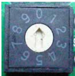
Fig. 13 Diagram of switch for timing closing function on three-phase electrical controller circuit board
